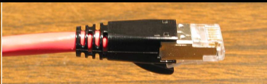
If used, align the strain relief grommet and push it over the terminated plug body. Snap it in place.
