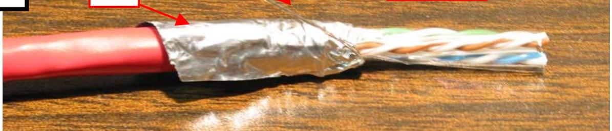
Fold the foil shield and drain wire back over the cable jacket.
