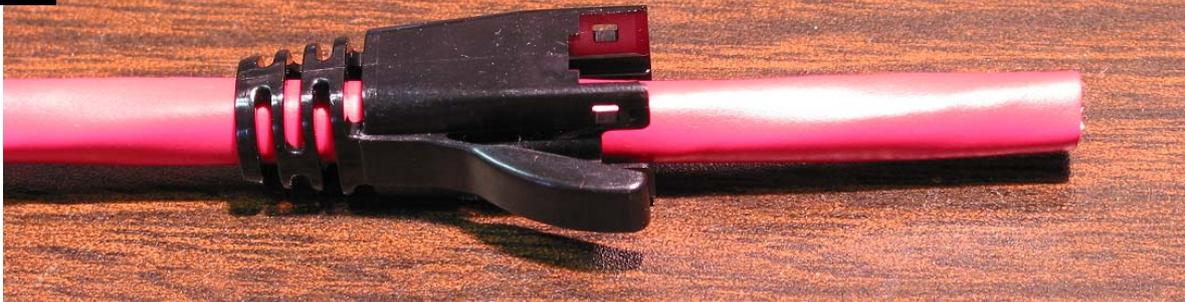
Cut cable to length. If you are using a strain relief grommet, slide it over the cable. The larger ends should be facing outward, toward the plug end of the cable.
