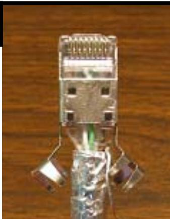
Wrap the drain wire around the foil near the wire aligner. Keep the orange pair to the left. Push the assembled wires, loadbar, and plastic wire aligner into the plug body subassembly. The plug latch tab should be facing away from you. Firmly push the plug until the wires come in contact with the front inside surface of the plug.
