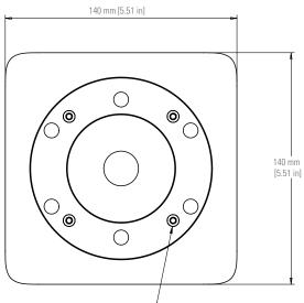
Threads for camera attachment M4 x 4
