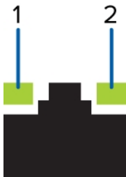
Figure 3: (1) Link LED. (2) Connection Status LED.
