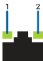
Figure 5: (1) Link LED. (2) Connection activity LED.
