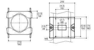
ES-HD-MNT-POLE-SM Small pole mount with dual camera adapter. Finish Epoxpolyester powder painting, RAL 9002 color Mounting Stainless steel screws Hardware Weight 0.9 kg (2.2 lb) Pole 65mm to 110 mm (2.5" to 4.3") Diameter Load Rating 30 kg (60 lb)
