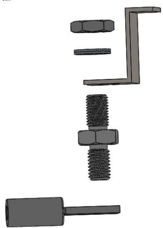
Figure 8. Retaining clip order
