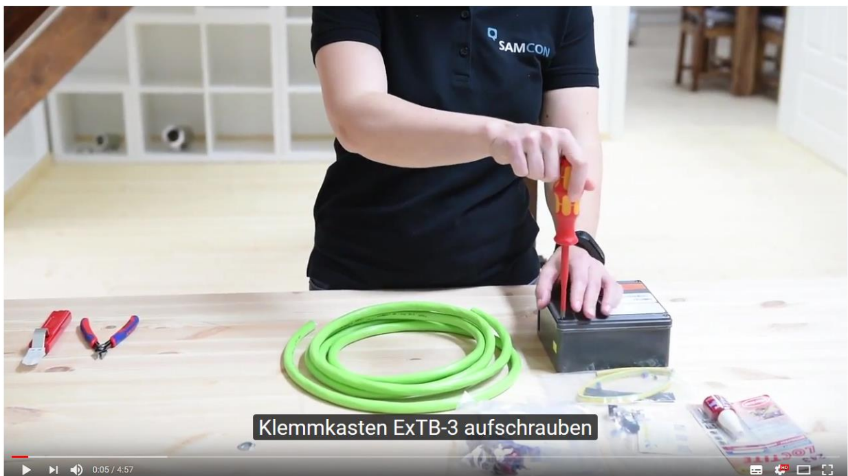
Fig. 5-3 Video Tutorial ExTB-3: Screw on the terminal box ExTB-3
