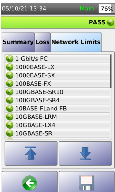
Figure 3 - Network Limits reports all networks that can be supported by the cable based on test results
