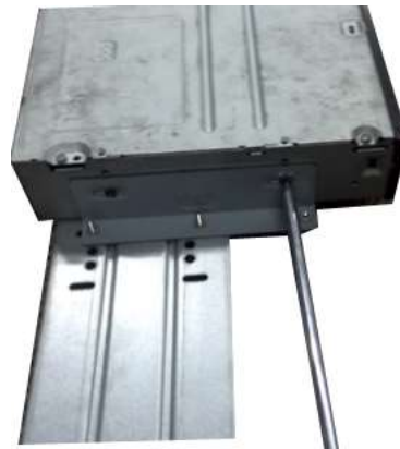
⑥ User screwdriver to fix the screws.
