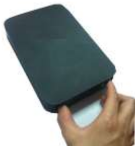
① Draw out the HDD bracket
