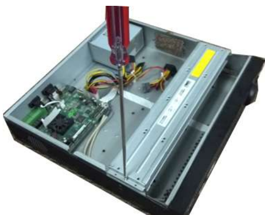
① Open top cover and then remove the HDD bracket
