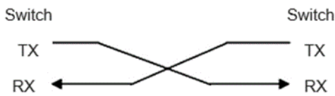
Figure 7-1 Optical Cable Connections
