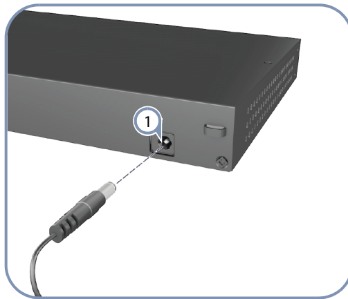
Figure 5: Connecting DC Power
