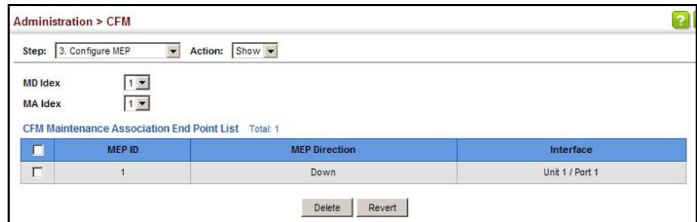
Figure 308: Showing Maintenance End Points
