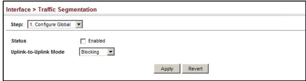
Figure 71: Enabling Traffic Segmentation
