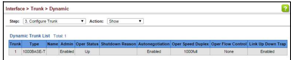
Figure 54: Showing Connection Parameters for Dynamic Trunks
