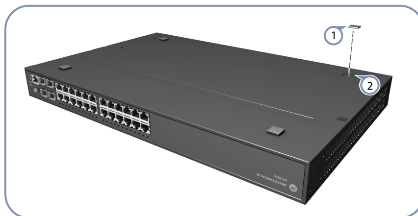
Figure 6: Attaching the Adhesive Feet
