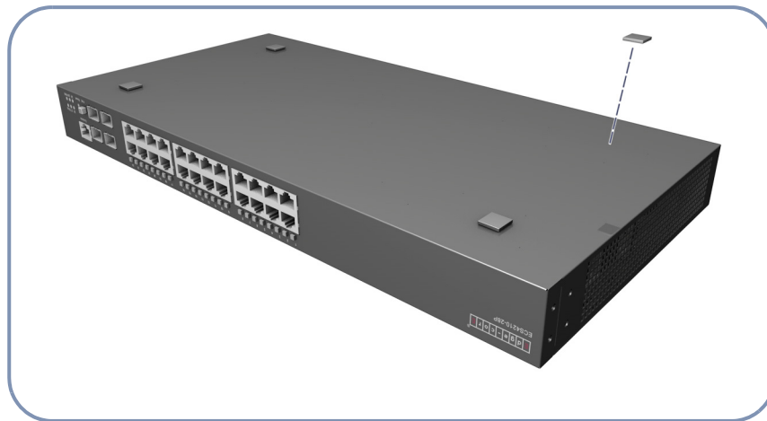
Figure 10: Attaching the Adhesive Feet
