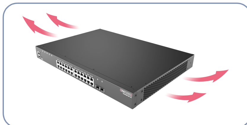
Figure 10: Switch Cooling (ECS4510-28T)
