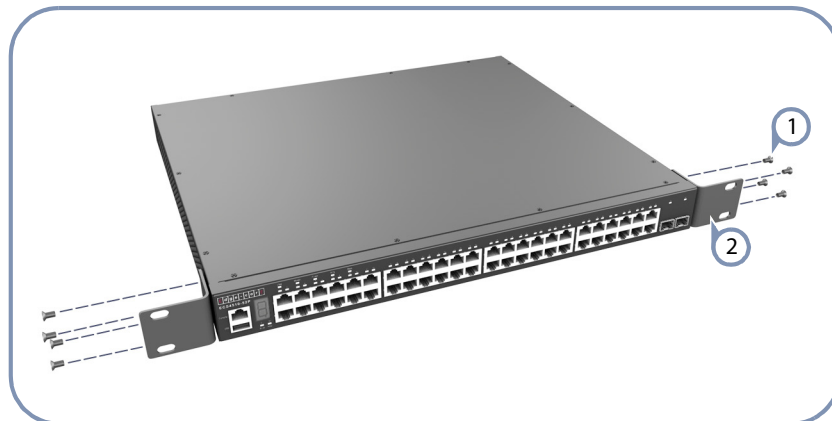
Figure 11: Attaching the Brackets
