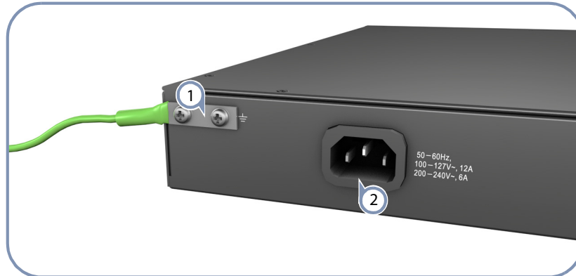
Figure 4: Connecting AC Power
