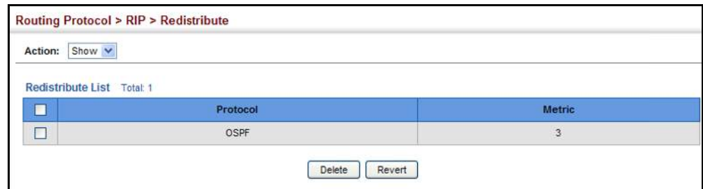
Figure 441: Showing External Routes Redistributed into RIP
