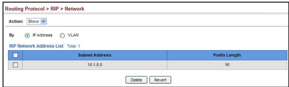
Figure 435: Showing Network Interfaces Using RIP
