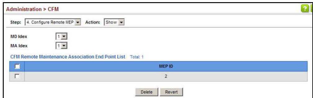
Figure 315: Showing Remote Maintenance End Points
