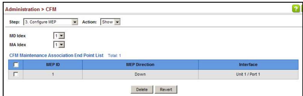
Figure 313: Showing Maintenance End Points
