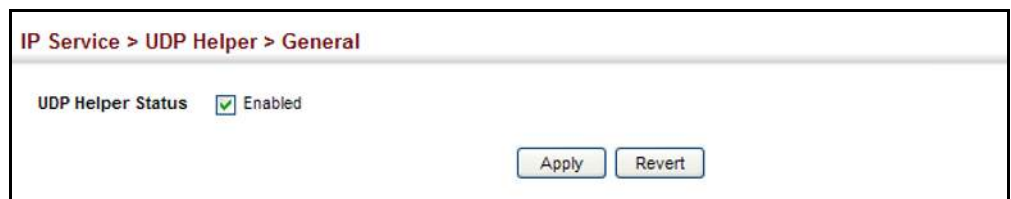
Figure 432: Enabling the UDP Helper
