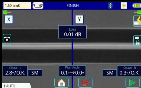
Splice loss with large cleave angle : 3 < \theta < 5 degree
