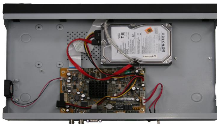
Figure 2-4 Fix Hard Disk
