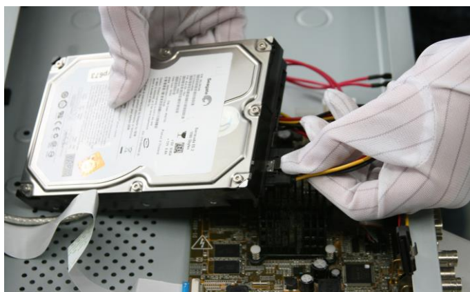
Figure 2-3 Connect Power Cable
