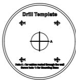
Figure 2-12 Drill Template of the Junction Box
