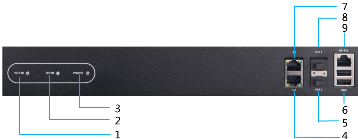
Figure 2-4 Front Panel of DS-6916UDI(B)
