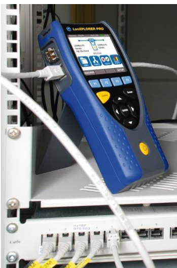
Figure 5: In-line Ethernet tester speed network troubleshooting
