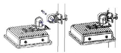
Attach the articulation pole to the mount base articulation using M8x90 bolt, nut and washers.
