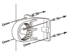
Fix the mount base to the wall using wood / gyprock screws.
