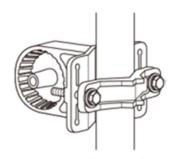
Mounting For Pole Larger than 1.5"(35mm) and Less Than 3" (80 mm)
