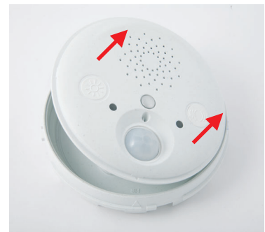
Remove the back of the housing
