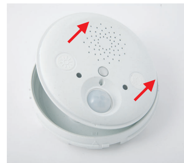
Remove the back of the housing
