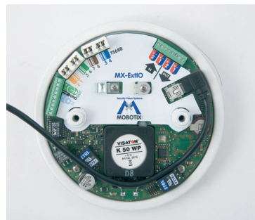
Insert USB plug Properly guide the cable
