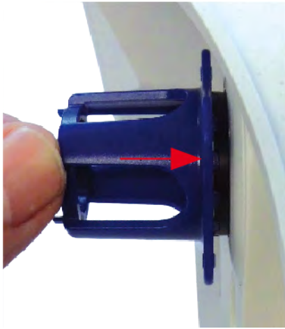
Fig. 57: Push hard to insert lens protection glass and turn to lock
