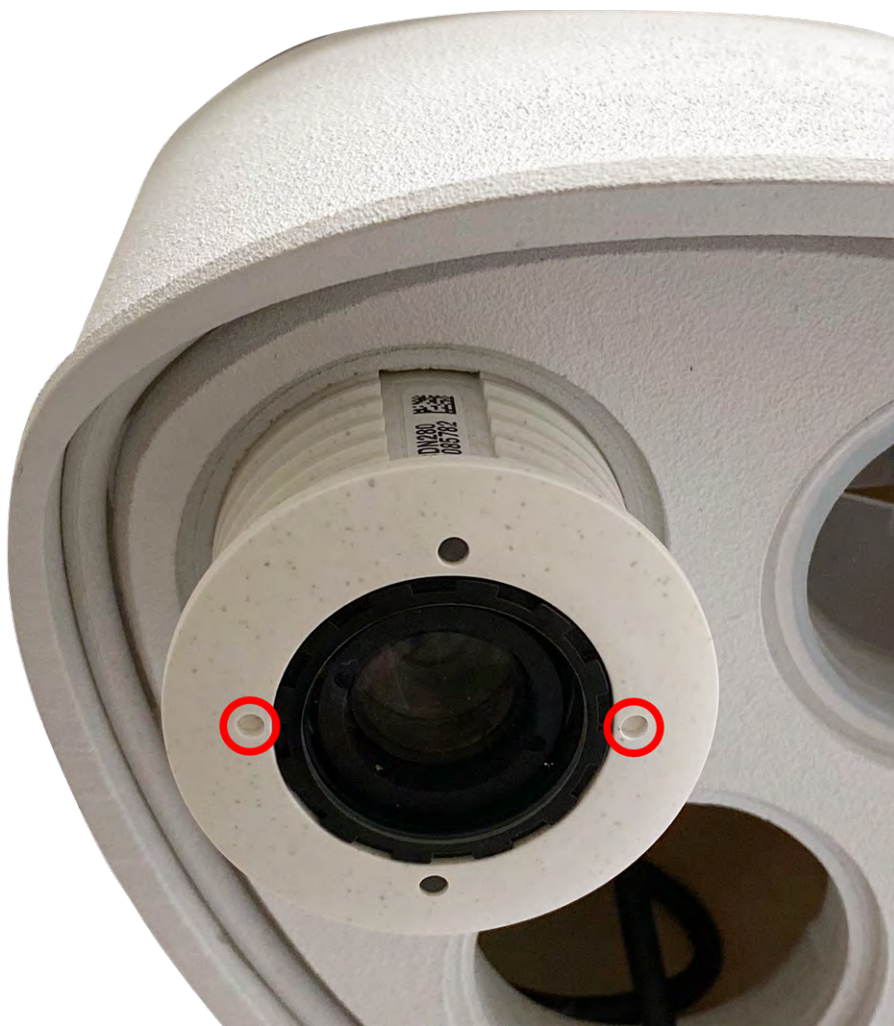
Fig. 24: Remove sensor module from the module housing
