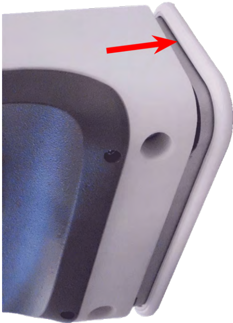
Fig. 41: Press camera onto mounting plate
