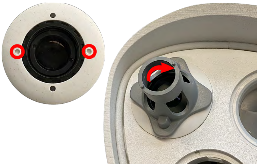
Fig. 30: Lock the sensor module
