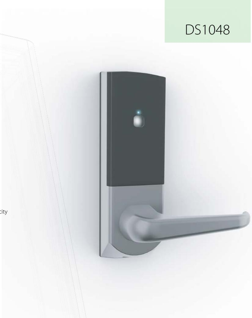
Easyprox nano is a Net2 access control unit in a door handle. It combines a wireless access control unit and a reader in one. Net2 is a PC based security system for controlling access through doors. Net2 allows users to be given access to particular areas at certain times. Because the system is networked, all administration can be done from a central point.
