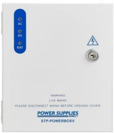
This boxed power supply provides a 12Vdc output for powering access control products such as keypads, maglocks, electric releases, solenoid bolts, etc. Its battery back-up feature enables continuous power during mains failures when fitted with an optional lead-acid battery.
