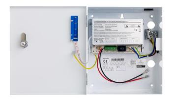
This boxed power supply provides a 12Vdc output for powering access control products such as keypads, maglocks, electric releases, solenoid bolts, etc. Its battery back-up feature enables continuous power during mains failures when fitted with an optional lead-acid battery.
