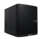
Typically, at least 48 network cameras can be connected to each NVR, which are supplied preinstalled with Wavestore's Video Management Software (VMS). Housed in a compact mini-tower case, suitable for desktop or shelf mounting, PT-Series NVRs can accommodate up to 4 x 3.5" hot swappable hard drives to provide up to 40TB of storage. This can deliver 45 days continuous real-time recording from 48 Full HD cameras in a typical installation\*\*.
