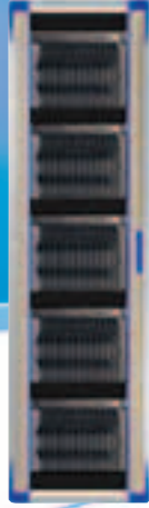
5 x 7U Blade Boxes \Sigma 15KW
